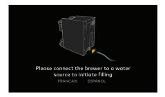
The brewer will automatically fill the internal hot water tank with water and then the water will be heated. This will take about three minutes. During the heating period, "Brewer is heating" will be displayed on the touchscreen.
